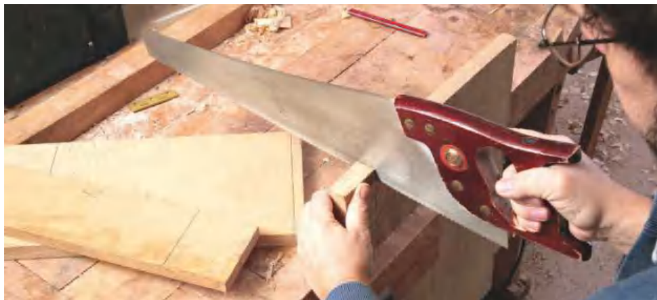
▲ Pic.15 Big saws like this can be very accurate but they tend to be used less by furniture makers nowadays while small hand saws are essential for fine work
